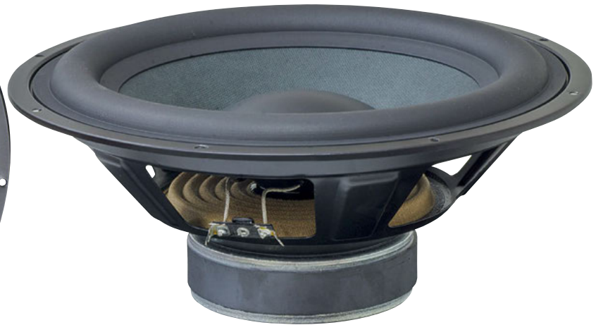
The 25-cm diameter woofer is of traditional construction, with a 38-mm voice coil, pressed sheet metal basket and ferrite magnet with decompression hole.
