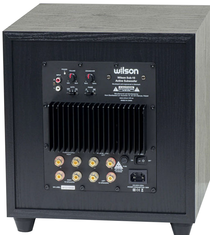
The rear panel houses stereo RCA connections and high-level signal terminals. Controls rely on two potentiometers to adjust cutoff frequency and level while phase can only be inverted with a selector switch. The amplifier's heatsink appears well sized.
